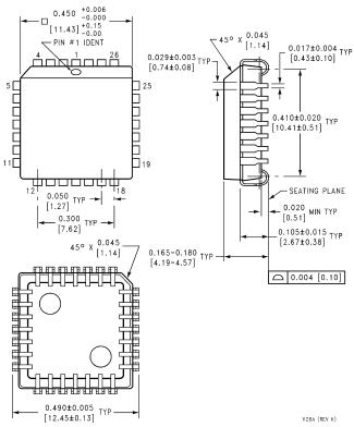
Molded Chip Carrier (V)
