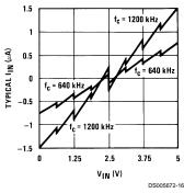
FIGURE 6. Comparator  $I_{IN}$  vs  $V_{IN}$  ( $V_{CC}$ = $V_{REF}$ =5V)
