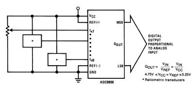
FIGURE 9. Ratiometric Conversion System
