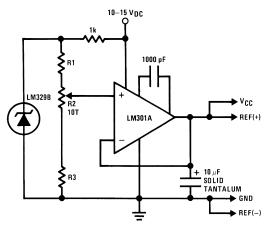
FIGURE 12. Typical Reference and Supply Circuit
