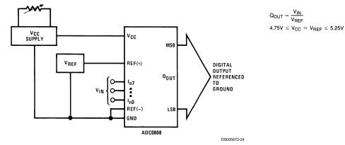
FIGURE 10. Ground Referenced Conversion System Using Trimmed Supply
