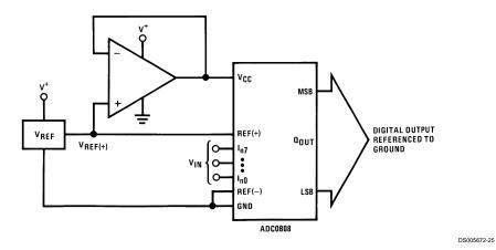
$\begin{aligned} Q_{OUT} &= \frac{V_{IN}}{V_{REF}} \\ 4.75V &\leq V_{CC} = V_{REF} \leq 5.25V \end{aligned}$
